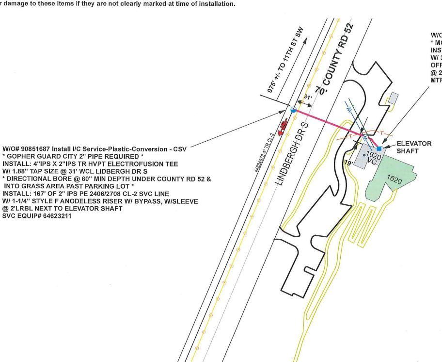
W/O# I/C Install SmVol Gas Meter - CSV \* MOUNT METER ON POST NEXT ELEVATOR SHAFT \* INSTALL: 425TC OSM ERT'D METERSET (CL-2 398CFH) W/ 3/4" X 1" 1813C REG @2#PSI, W/ 3/8" ORIFICE OFF 1-1/4" STYLE F ANODELESS RISER W/BYPASS, W/SLEEVE @ 2'LRBL NEXT TO ELEVATOR SHAFT MTRSET# 15272386
