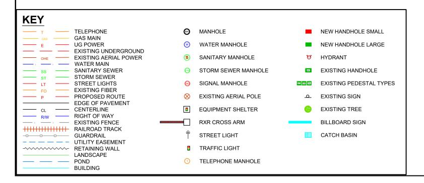
HH# = HAND HOLE NUMBER = 30"x48"x48" HAND HOLE = 24"x36"x24" HAND HOLE FOSW = FRONT OF SIDE WALK BOC = BACK OF CURB EOP = EDGE OF PAVEMENT ORWL= OFF ROAD WHITE LINE EOGR = EDGE OF GRAVEL ROAD BOW= BACK OF WALL BOSW = BACK OF SIDE WALK
