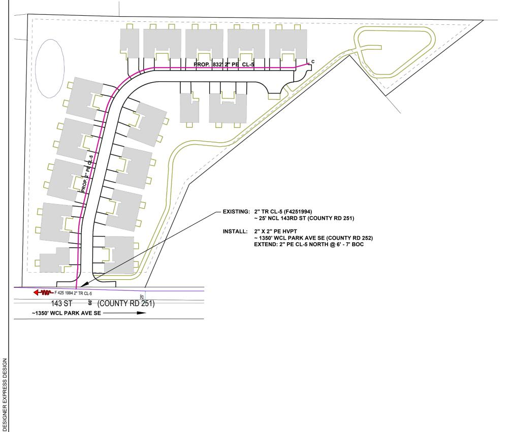
NOTE: BORE ALL PAVED STREETS AND DRIVEWAYS Minimum depth requirements for crossings of state highways and county roads is 60". Minimum depth requirements for crossings of city streets and township roads is 48". Minimum depth for parallel installations on state highways and county roads is 36". Minimum depth for parallel installations on city streets and township roads is 30". All steel pipe welds to be coated with 2 part epoxy.
