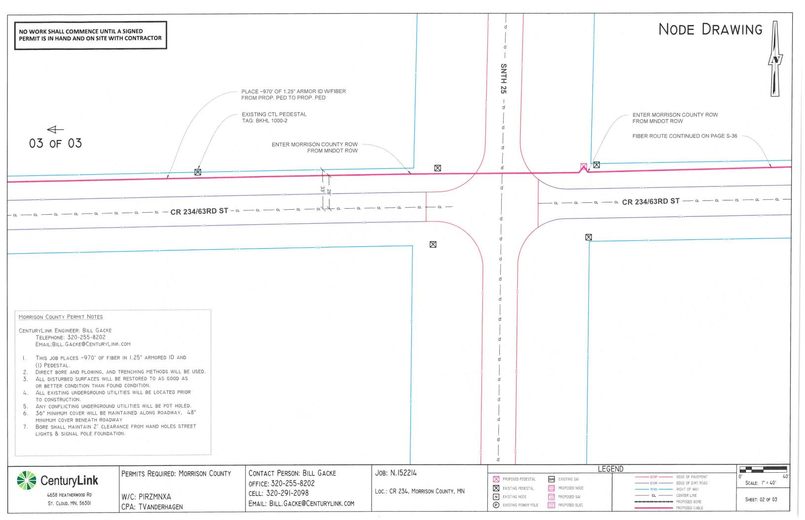
NODE DRAWING NO WORK SHALL COMMENCE UNTIL A SIGNED PERMIT IS IN HAND AND ON SITE WITH CONTRACTOR PLACE ~970' OF 1.25" ARMOR ID W/FIBER FROM PROP. PED TO PROP. PED DIRECT BORE 50' UNDER CR234 FIBER IN 1.25" ARMORED ID MIN DEPTH 48" X ca - CR 234/63RD ST - ca -END PROPOSED 48 FIBER RUN @ PROPOSED PEDESTAL RT SAI → 02 of 03 PROPOSED CTL PEDESTAL LAT: 45.854141° LONG: -94.096092° SEE N.191250 NODE DETAILS
